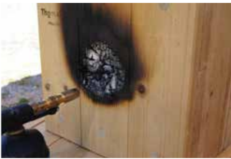
Test pieces of the solid timber element of the outer wall for HOLZ100 after 60 minutes subjected to a direct flame, at a temperature of approximately 900°C
